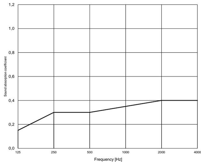
Practical sound absorption coefficient, weighted sound absorption coefficient, and absorption class according to EN ISO 11654:1997:
