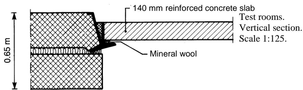
Test opening with standard floor.
