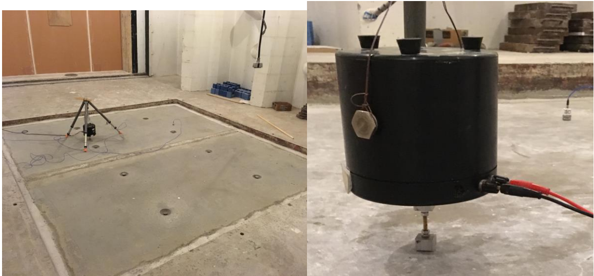
Figure 3 Mounting of exciter on test deck for the structural reverberation time.
