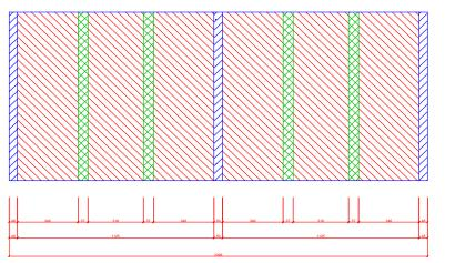
Underside of SL-decks - attachment zones
